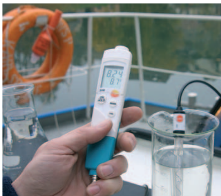
Automatic temperature compensation with external probes with temperature sensor
