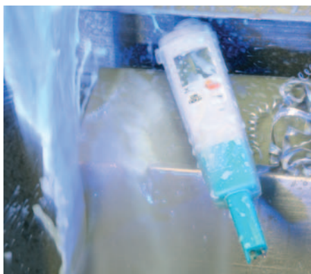
The "TopSafe" case protects in tough industrial conditions
