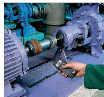
rpm measurement on shafts
