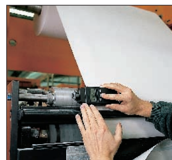
Mechanical rpm measurement on a roller
