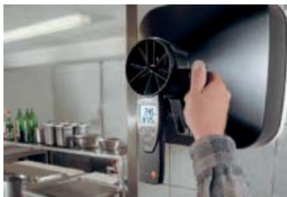
testo 417, e.g. for monitoring the exhaust air at a wall-mounted ventilator
