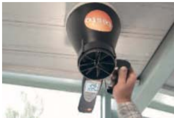
testo 417, e.g. for monitoring the air input at a plate ventilation outlet
